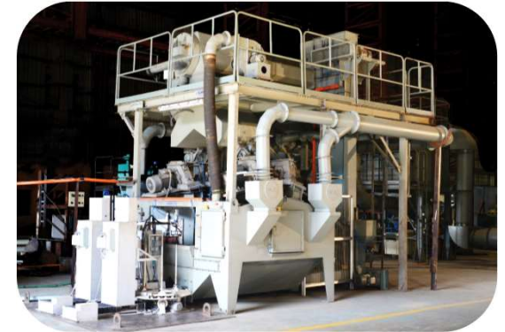
CNC shot peening for clutch plates
